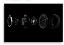
A pre-tilted driver matching the ear cup's natural angle directs the sound straight into the ear canal. This means much less of the coloration that can occur when sound reflects off the outer ear, together with a more realistic soundstage and enhanced comfort.
