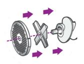
The knife can only be assembled correctly on the feeding screw
