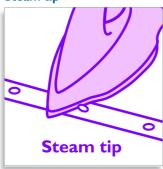
The unique steam tip combines a particularly pointed front of the soleplate with special elongated steam slots in the tip, to reach right into the smallest and most difficult areas for the best ironing results.
