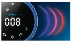
See the real-time air quality in your home at a glance. The display shows the level of allergens, gases and PM2.5 in numerical form, as well as with an intuitive color ring.
