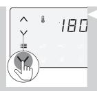
**6** Press the temperature up or down button to choose the needed temperature.
