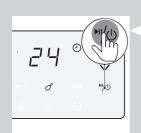
2 Press the On/Off button again to turn on the device.
