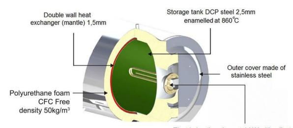
Electric heating element 4 kW with adjustable safety thermostat (30°- 80°C) and magnesium bar Ø22x300mm for anodic protection
