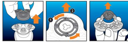
1. Open the shaver by pressing the "release" button; 2. Remove the retainer by turning the lock anticlockwise; 3. Take out the old shaving heads and carefully insert replacements; check that the heads align exactly in the setting; 4. Replace the retainer and secure it by turning the lock clockwise; 5. When you close the shaving head properly, you will hear it click into place.
