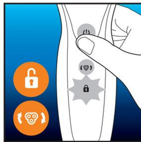
After replacing the shaving heads, you can reset the replacement reminder by pressing the on/off button for more than 7 seconds. Otherwise, the replacement trigger will turn off automatically after 9 successive shaves.
