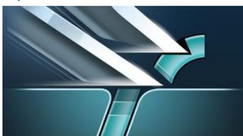
The dual-blade system built into our electric shaver lifts hairs to cut comfortably below skin level for a closer shaving experience.
