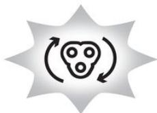
The latest Philips shavers have an inbuilt replacement reminder in the form of a shaving unit symbol. This symbol will light up and indicate when to replace the shaving heads.
