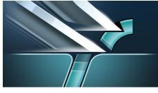
The dual-blade system built into our electric shaver lifts hairs to cut comfortably below skin level for a closer shaving experience.
