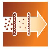
The two stage filtration system ensures that, once inside, the dirt cannot escape again. The first filter blocks most of the dirt, while the second filter traps the finer dust particles.
